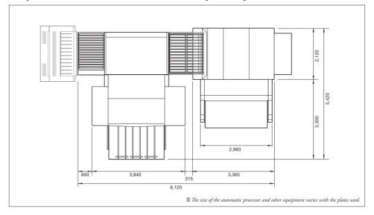
■ Layout for PlateRite Ultima 16000N with MA-L16000NII (six-cassette autoloader type) [units: mm]
